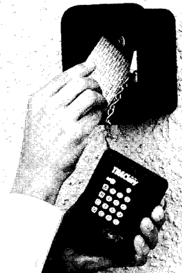
TRACkey provides power to activate most locking devices and to record each access
